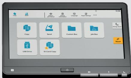
*The 10.1-inch operation panel with its simple and intuitive user interface, for quick and easy use of the device.*
